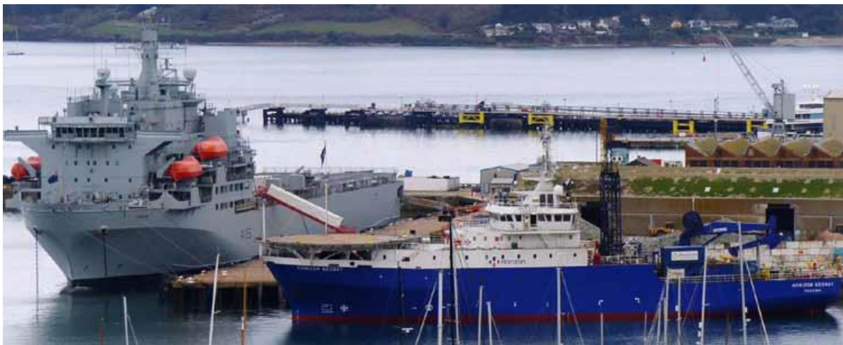
Horizon Geobay (ex Salvanguard ex Dahlia ) a DP2 multipurpose vessel coming alongside at Falmouth UK after a period in drydock. Vessel built in 1978 and now under Panamanian flag, GT3502T, DWT 2404T, 87m x 15.68m. Also alongside is seen the RFA Argus .
